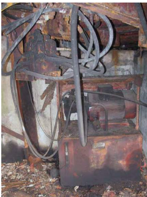
Plate 25.5: Building 25: hydraulic reservoir and pump beneath the conveyor, view to the east
