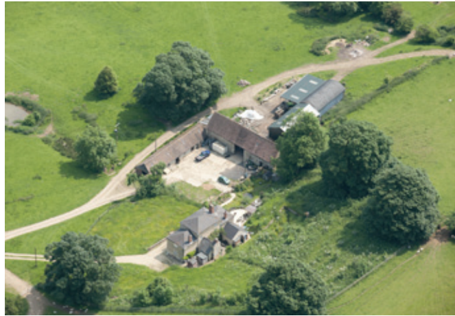
A mid-18th century regular courtyard L-plan farmstead located on the slopes of Bredon Hill. The farmstead comprises a threshing barn, with its large central doorway, attached to single-storey cattle housing. Photo © English Heritage NMR 27761/031
