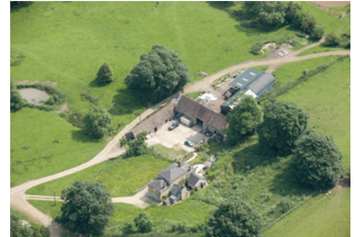
A mid-18th century regular L-plan farmstead, constructed of coursed stone rubble, on the slopes of Bredon Hill. The 2nd Edition Ordnance Survey map records a covered yard, now lost. The L-plan comprises a threshing barn, with its large central doorway, attached to single-storey cattle housing. Photo © English Heritage NMR 27761/031
