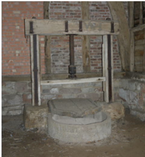
LEFT: A cider mill, around which a horse pulled the millstone for crushing fruit fed into the trough. Photo © Jeremy Lake
