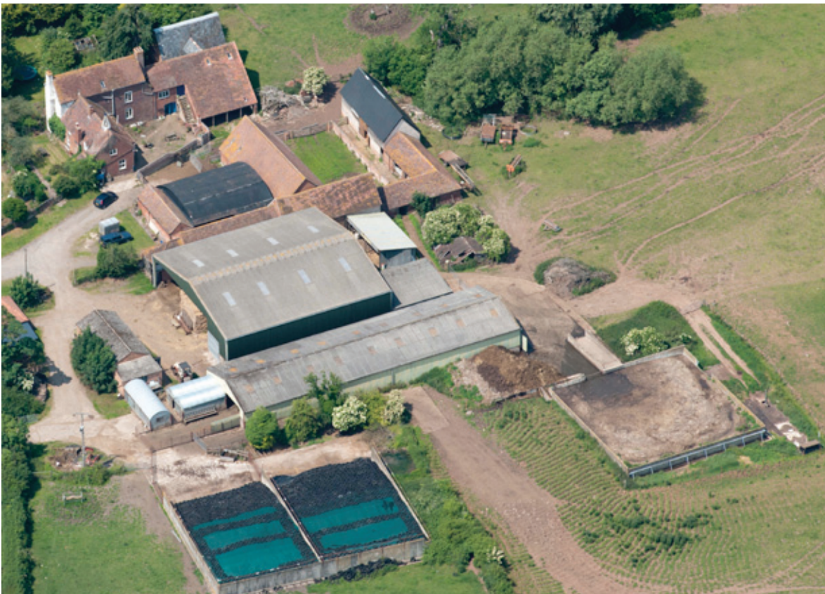
Isolated farmstead with traditional buildings, arranged around two yards, and 20th century wide-span multi-purpose sheds (Central Worcestershire Plain Farmstead Character Area). The extant traditional farm buildings date from the 17th century to the 19th century and include a timber-framed threshing barn and red brick granary, cart shed, cow house and hop kiln. Photo © English Heritage NMR27763/018
