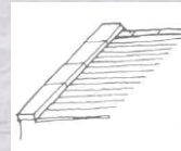
Coping at gable
