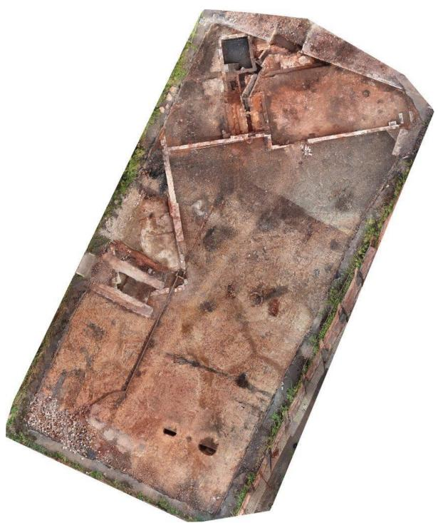
Plate 2: Aerial photograph of Area 2, showing the southern wall of the enamelling works and the flues and chambers of the furnace in the north
