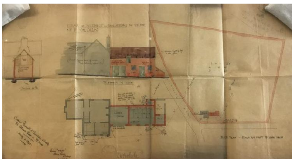
Plan of cottage residence, plus ancillary buildings including a coach house, stables and pig sty, at the Woodrow Farm Small Holdings Estate (Plot 25), for Mr B. Waldron. Although extant it was not possible to obtain photographs of this residence during field survey. Surrounded by construction fencing the building, which was last sold in 2019, appears to be undergoing renovation.
